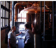
SENSORS IN THE KETTLES MONITOR VOLUME AND TEMPERATURE, WHERE SIMPLE SUGARS AND PROTEINS FROM MALT ARE EXTRACTED TO ACHIEVE SPECIFIC GRAVITY LEVELS.
